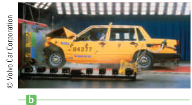
Figure 6.4 (Example 6.2) (a) This car's momentum changes as a result of its collision with the wall. (b) In a crash test (an inelastic collision), much of the car's initial kinetic energy is transformed into the energy it took to damage the vehicle.
