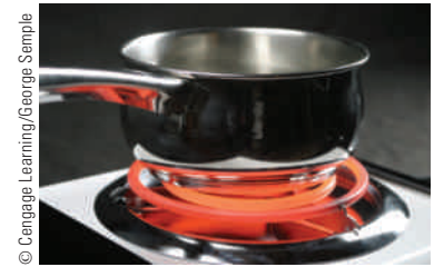
Figure 11.4 Conduction makes the metal handle of a cooking pan hot.
