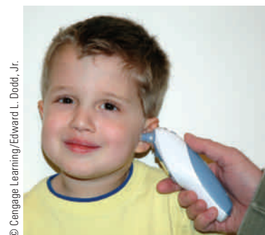
Figure 11.14 A radiation thermometer measures a patient's temperature by monitoring the intensity of infrared radiation leaving the ear.
