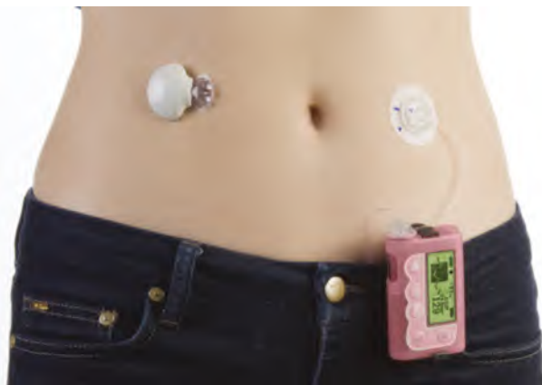
FIG. 14.7 MiniMed paradigm REAL-time revel system. The insulin pump is small and can be worn under clothing or on a belt. It delivers insulin through a tube or cannula (infusion set) that is inserted into the subcutaneous (SC) tissue. The pump can be disconnected for bathing, swimming, or changing clothes. A small sensor for glucose is inserted into the SC tissue using an automatic insertion device. Sensor data are sent to a transmitter that is attached to the skin with a waterproof adhesive patch. The transmitter sends data to the insulin pump using wireless technology. The sensor and tube (new tubing) from the pump must be relocated every 3 days to minimize the risk of infection obstruction of the tube. (Courtesy of Medtronic, Diabetes, Minneapolis, MN.)
