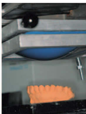
Fig. 30.13 A. A traditional vacuum suction machine used to make custom made mouthguards. At top there is a heating element; the stock plate is sandwiched in a jig right underneath the element. The cast is placed on a perforated plate and care must be taken that it is as much in the center as possible. When the stock plate heats up it will start to droop, so care must be taken not to overheat it because that will result in too thin mouthguard. Most commonly used EVA materials should droop about 2–2.5 cm (3/4–1 inch) before being sucked down on the cast. C. The plate needs to completely cool down on the cast before it is removed from the cast.
